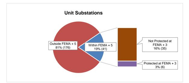
Figure 15 Current protection level of Con Edison unit substation assets relative to FEMA + 3'
