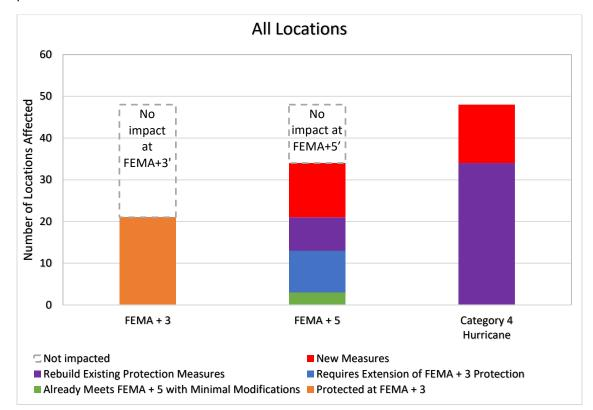
**Figure 9** Current protection level of Con Edison assets relative to FEMA+3' flood, FEMA+5' flood, and potential Category 4 hurricane surge scenarios, and potential for extending existing protections.
