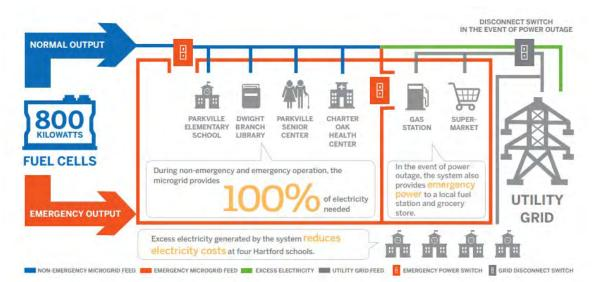
**Figure 17** Diagram of the microgrid operations during normal and emergency operations. Source: Constellation Energy
