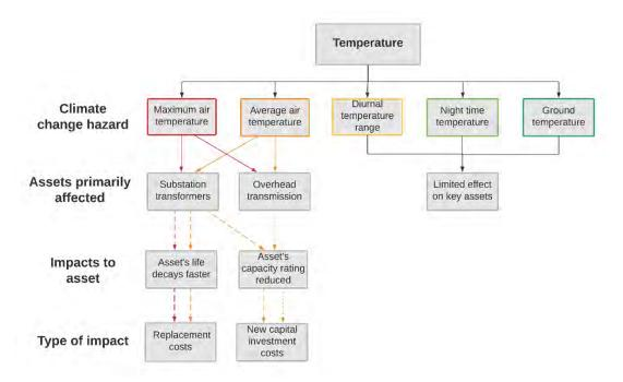
Vulnerabilities to temperature can be inherent in the design of individual components of Con Edison's system (physical vulnerabilities) or they can be introduced in the ratings that dictate the appropriate operations of a particular system that is made up of several components (operational vulnerabilities). Figure 9 provides a more detailed perspective on the relationship between design parameters and ratings, which provides context for the following sections.
