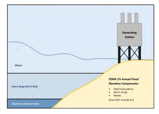
Figure 2 Elements of FEMA's 1% annual flood hazard elevation
