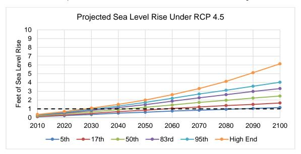
**Figure 11** Projected sea level rise (RCP 4.5) relative to 2000 under various percentiles. The black dashed line depicts the 1-foot sea level rise threshold from the current design standard.
