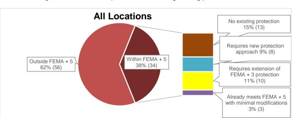
**Figure 14** Current protection level of Con Edison substation assets relative to FEMA + 3' and FEMA + 5' design standards, and the potential for extending existing protections
