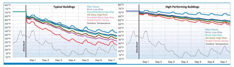
Figure 20 Modeled indoor temperatures for typical and high-performing buildings during an extended winter power outage (Urban Green Council, 2014).
