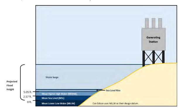
**Figure 7** Illustration of the components of Con Edison's projected flood height (storm surge, sea level rise, and tides above mean lower low water)
