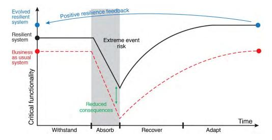
**Figure 14** The "absorb" component of a resilient energy system minimizes the consequences of extreme events.
