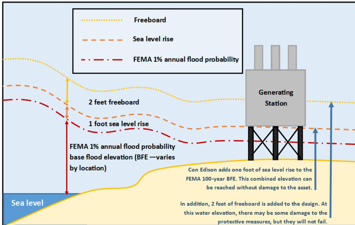
All Con Edison equipment within the FEMA + 3' flood zone is either designed to be submersible or is protected to that level by a barrier. For example, gas regulators must either have their vent line terminus above the FEMA + 3' elevation or have a vent line protector installed.<sup>6</sup>
