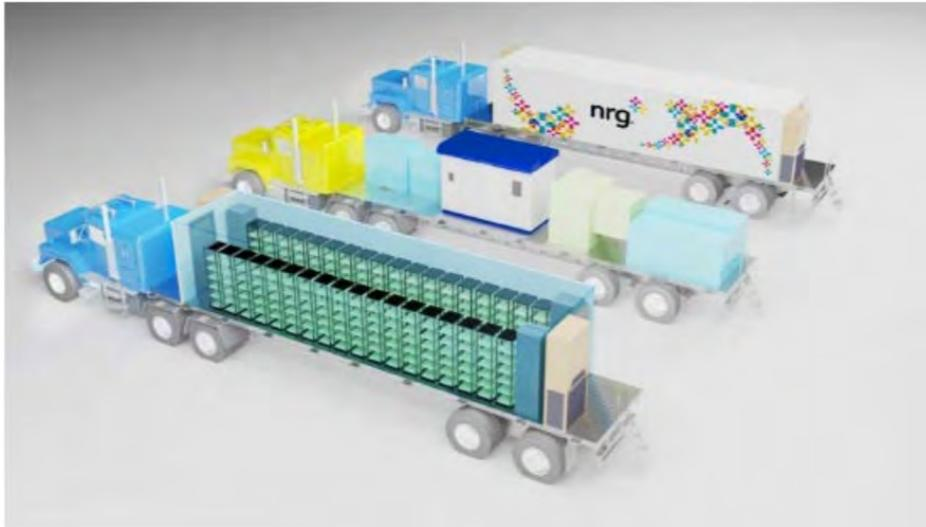
2. *Transportable Energy Storage System (TESS)*: Con Edison is working with a technology partner to develop and demonstrate a customer-sited, front-of-the-meter TESS (4 MW/4 MWh) within its service territory. The system will include lithium-ion batteries, a power conversion system unit, and an integrated thermal management system. If demonstrated to be a success, the trailer-mounted system could take the place of mobile diesel systems.
