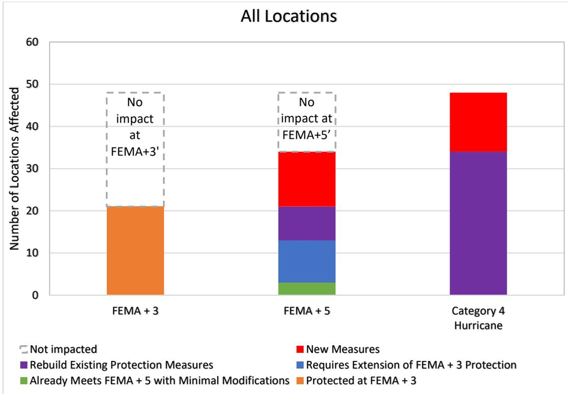
The Study team determined that, exposed to a Category 4 hurricane storm surge, 41 and 21 unit substations would require rebuild of existing protection measures and new protection measures, respectively (Figure 10). Fewer unit substations are exposed with the FEMA +3' and FEMA + 5' floodplains than for a Category 4 hurricane.
