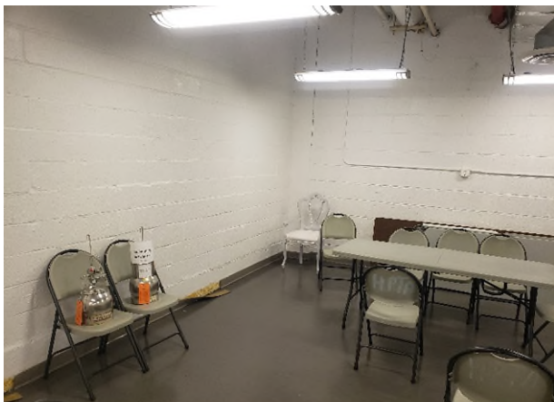
Photograph 41: HPL-Meeting Rm air sample and DUP-111820 air sample located adjacent to one another elevated from floor.
