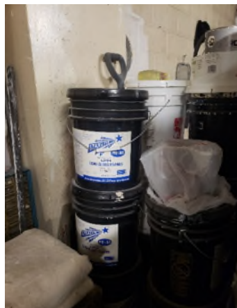
Photograph 24: Open latex enamel container in storage room 20 feet from HPL-Storage Rm air sample.
