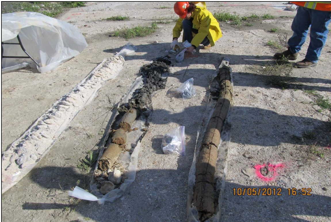
15. View of liner and sonic core barrel contents from soil boring DB-3, 5/10/12.
