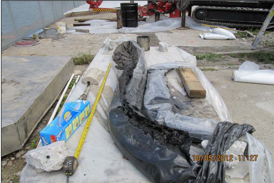
13. View of liner and sonic core barrel contents from soil boring DB-1, 5/10/12.
