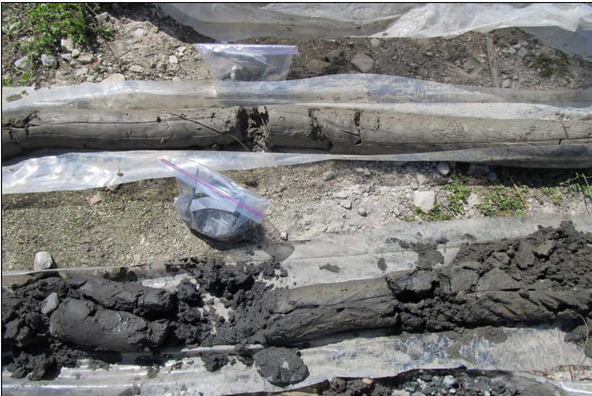
18. View of liner and sonic core barrel contents from soil boring DB-5, 5/11/12.
