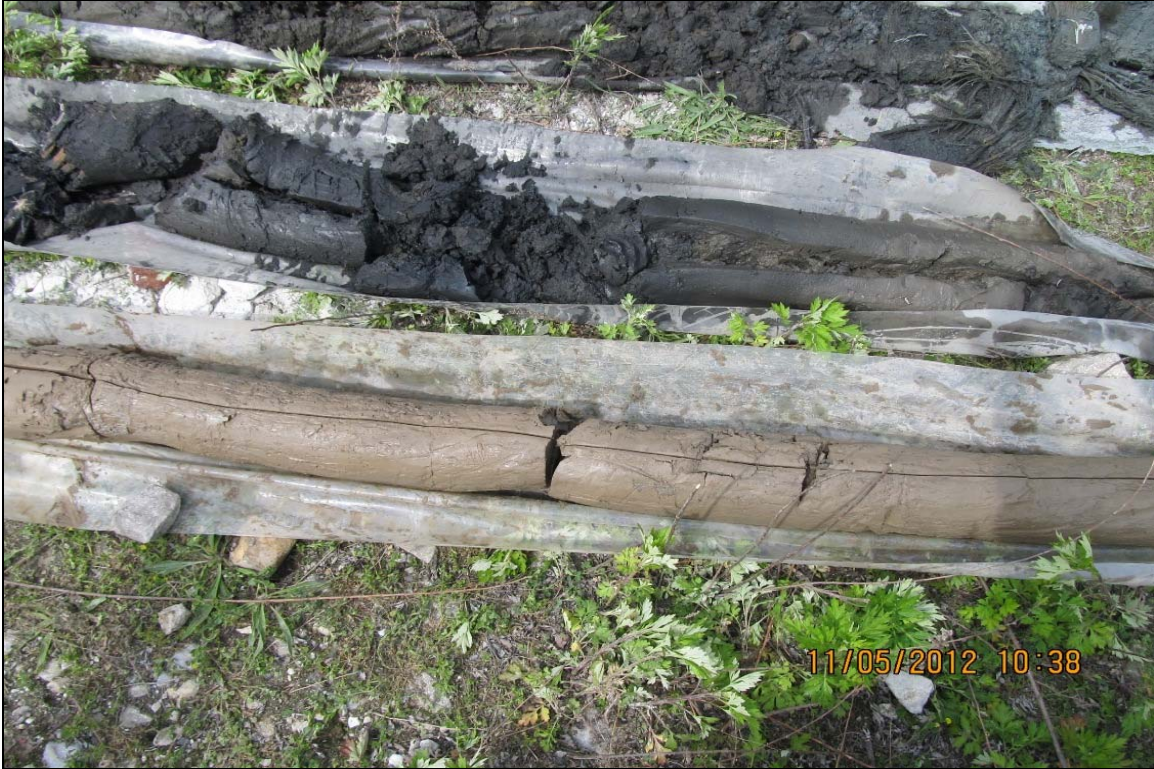
17. View of liner and sonic core barrel contents from soil boring DB-6, 5/11/12.
