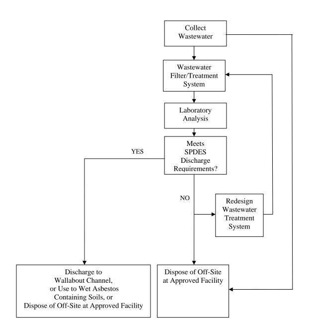
FIGURE 1: WASTEWATER FLOW DIAGRAM
